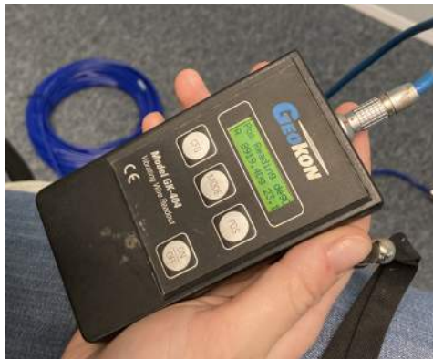
Figure 3.10: Portable readout device, model GK-404 VW, used the preliminary tests and load tests.
