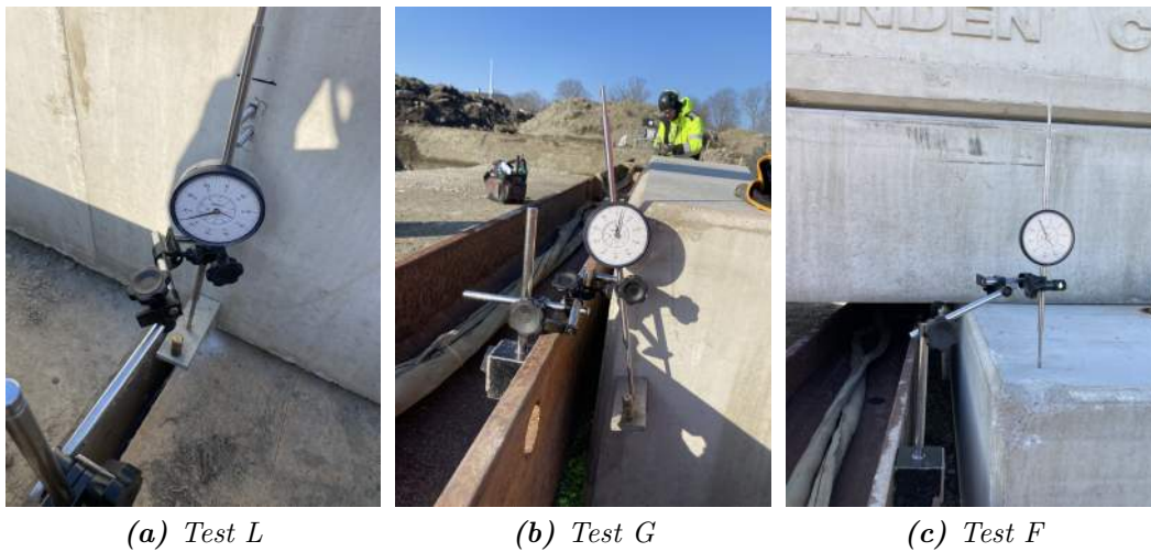
Figure 3.9: Dial indicator installation for the field trial.
