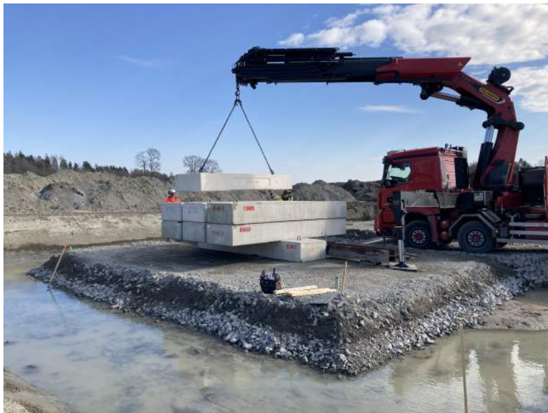
Figure 3.17: Photograph of test F as it is about to be loaded with the first weight of step 6.
